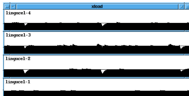
Figure 3.29: CPU load curves of four of the cluster of seven computers working in parallel. The dead times of individual units appear statistically during the closure runs of each generation, recognizable as small dips in the respective activity displays.
