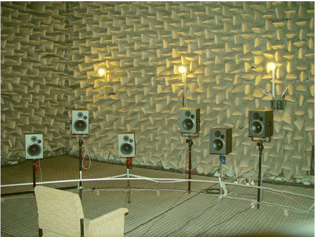
Figure 3.76: Experimental set-up in an anechoic room to generate a synthetic sound field. The problem addressed in this case is the subjective investigation of the apparent source width of an orchestra (following M. BLAU in KÖLTZSCH [Kö03])
