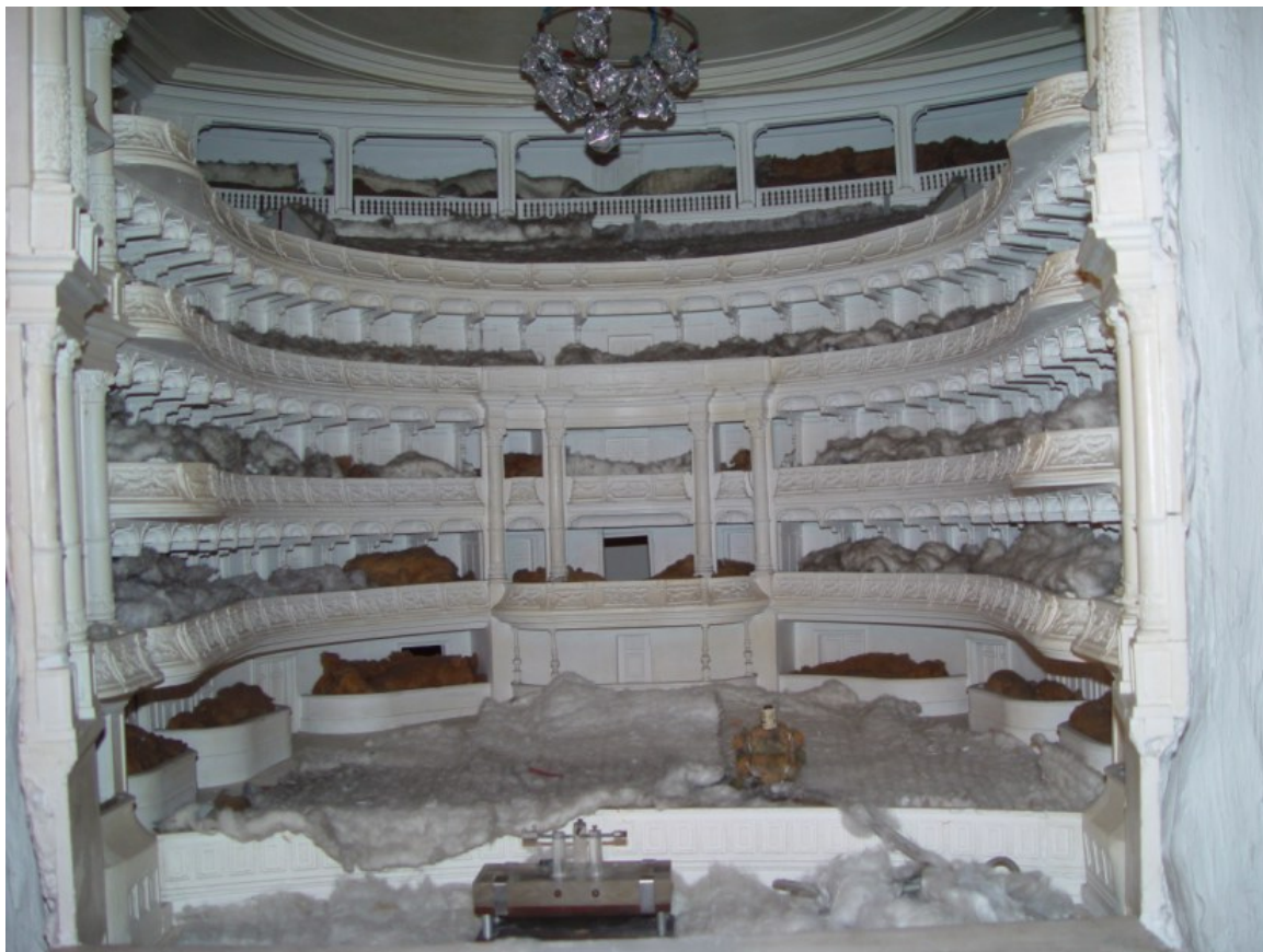
Figure 3.71: View into the auditorium of the model (1:20) of the historic Semper Oper Dresden. The model is equipped with absorbing material to simulate the audience. (photo: R. DIETZEL, TU Dresden)
