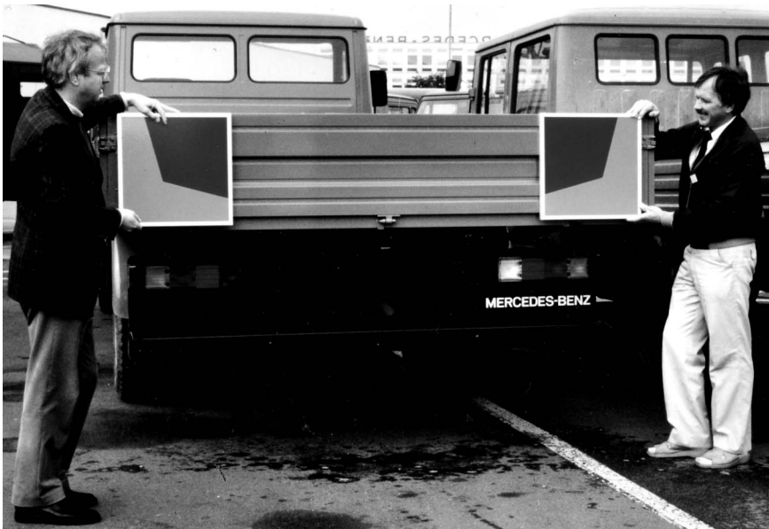
Figure 9–10. Retroreflecting rear marking plates.
