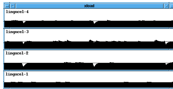
Abb. 4.14. CPU load curves of four of the cluster of six computers working in parallel. The dead times of individual units appear statistically during the closure runs of each generation.
