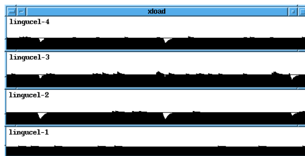
Figure 3.29: CPU load curves of four of the cluster of six computers working in parallel. The dead times of individual units appear statistically during the closure runs of each generation.
